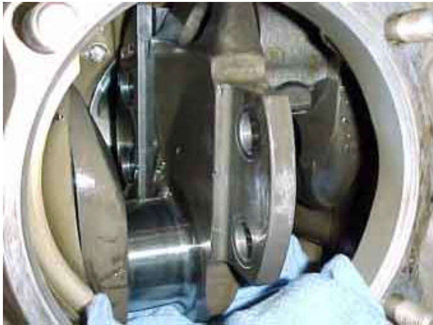
FIGURE 7. CRANKSHAFT COUNTERWEIGHT BLADE
