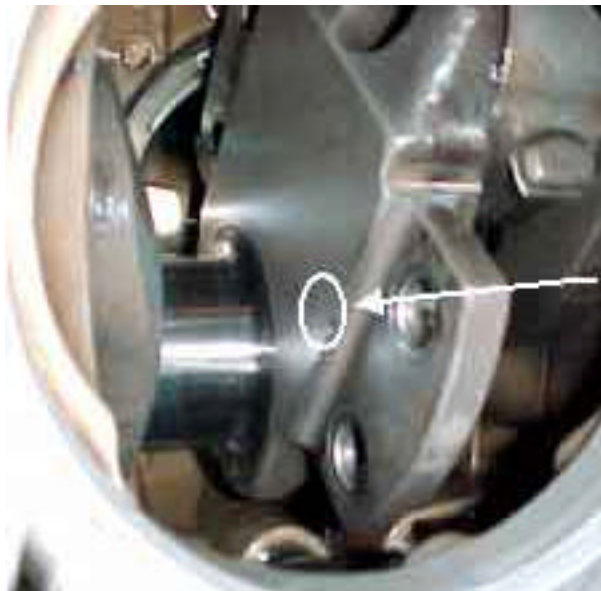
FIGURE 10. CRANKSHAFT IN INSPECTION POSITION #2 CRANKCHEEK CONNECTING ROD REMOVED
