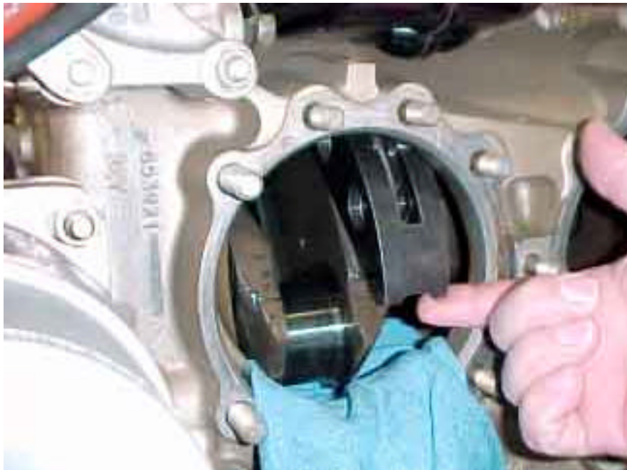
FIGURE 4. STARTING COUNTERWEIGHT THROUGH CYLINDER OPENING
