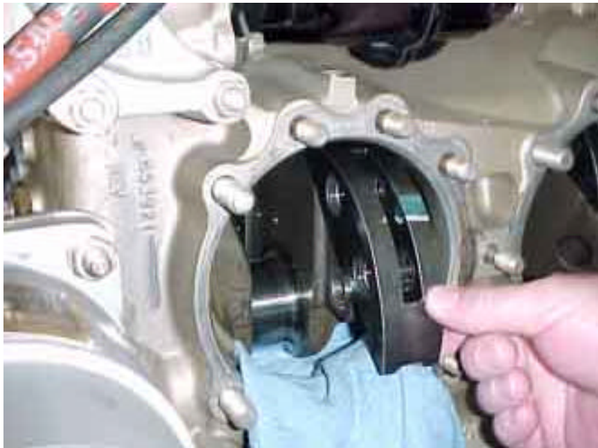
FIGURE 5. GUIDING COUNTERWEIGHT THROUGH CYLINDER OPENING
