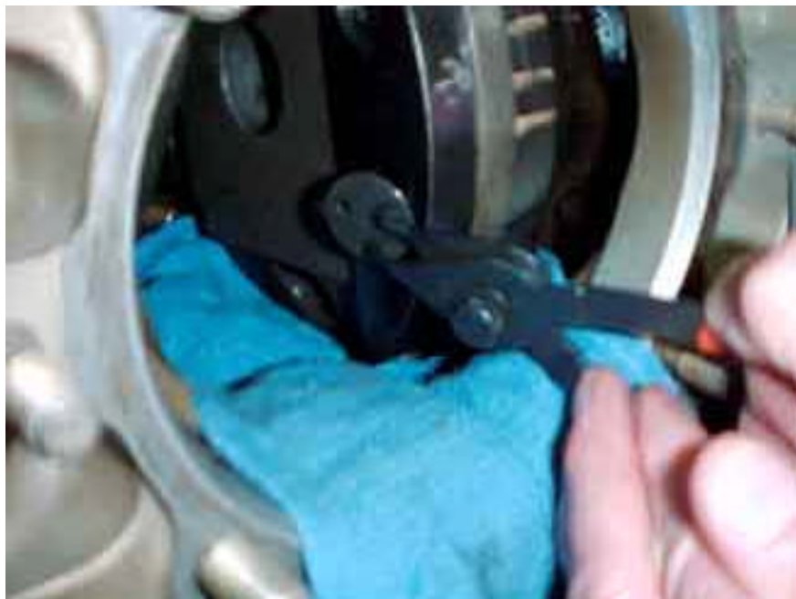
FIGURE 2. REMOVING COUNTERWEIGHT RETAINING PLATES
