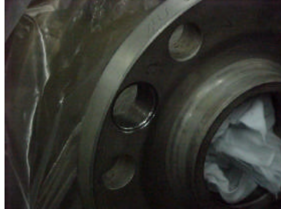
FIGURE 12 CORE SAMPLE HOLE AFTER CHAMFERING
